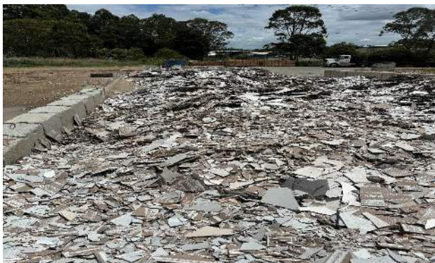
Plate 27 Rejected tile after firing for Concrush removal for repurposing
